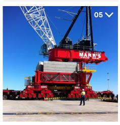
MAY 2013. Self-propelled modular transporter systems were used to load the 1,000 tonne M2480D tower crane onto the Barrow Island-bound super barge.
